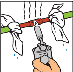
10. Heat with blow lamp.
