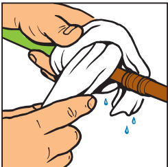
9. Wrap exposed plastic with a damp cloth.
